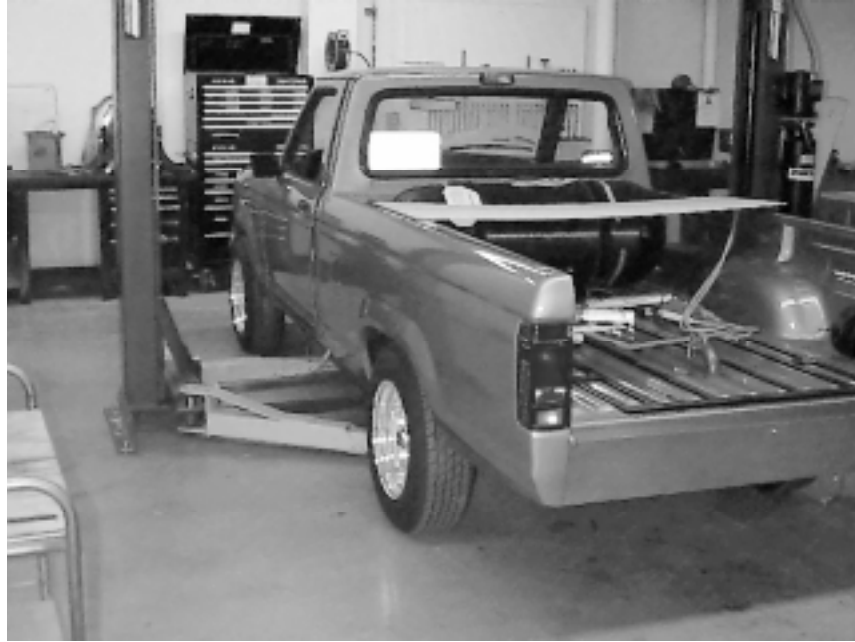
Hybrid-electric truck being outfitted with hydrogen-fueled auxiliary power unit, 1997.
